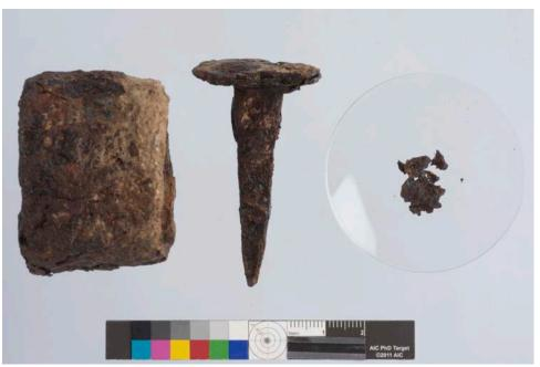
**Unstable; spalling bits; Untreated** was assigned in cases when untreated iron objects (with significant remaining burial soil) showed minor spalling (with fragments smaller than ∼1 cm), presumably as the result of one or more of the corrosion mechanisms described above.
