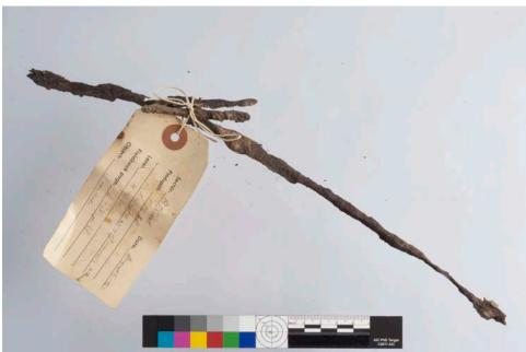
**Unstable; fragmentary; Untreated** was assigned in cases when untreated iron objects (with significant remaining burial soil) have been reduced to a fragmentary state (with fragments greater than ∼1 cm), presumably as the result of one or more of the corrosion mechanisms described above.
