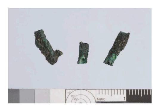
**Bronze disease?**; Untreated was assigned in rare cases when untreated objects (with significant remaining burial soil) had very small areas of potentially powdery corrosion but access to the area of the object was limited such that active bronze disease could not be confirmed with the naked eye. This category is not represented in the visual glossary.
